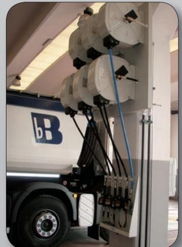
The electronic dosing system **AUTOMATIC FILLS** allows the dosage of different, preset quantities of a fluid lubricant.
